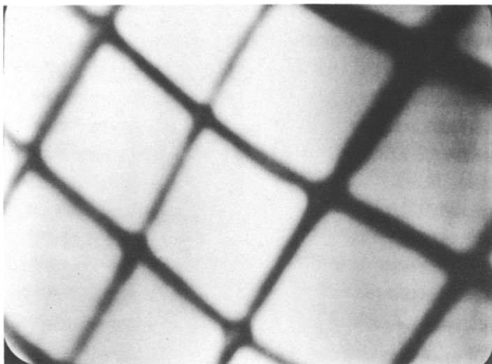
Figure 11 SAM image of a 100 mesh grid with a nominal spacing of 254 \mu\text{m} . This is to the same scale as the other SAM images.
