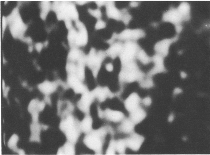
Figure 7 Scanning acoustic microscope (SAM) image of En8 steel (a) at 140 MHz. Dappled contrast is believed to be caused by scattering from grain boundaries.
