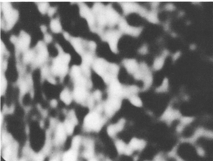
Figure 10 SAM image of diffusion bond (b) taken at 140 MHz. The specimen is rotated 45° from its alignment in Fig. 9, the vertical markings have also rotated.
