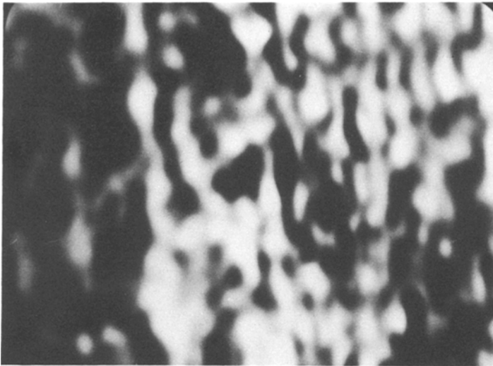
Figure 9 SAM image of diffusion bond (b) taken at 140 MHz. Several black vertical markings are visible, possibly caused by cylindrical voids on the bond interface.
